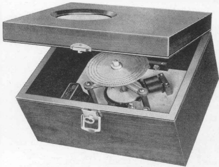
FIGURE 3. This synchronous motor is portable and connected to subsidiary amplifier circuits by a flexible cable. The disc makes use of transmitted light
